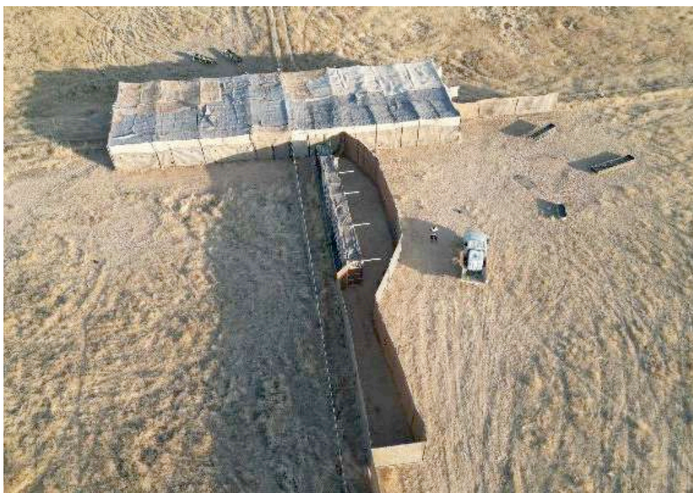
Fig. 6. Layout of capture pens and alley to Tamer Jr. as of October 25, 2025. Temporary fencing panels, shade cloth, and woven natural materials were used to completely enclose sections of the capture area and Tamer alley.
