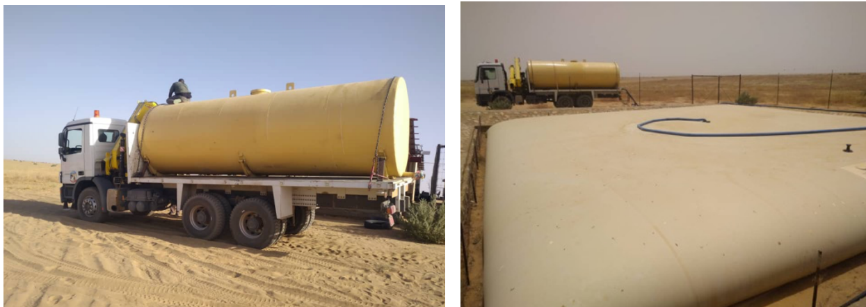
Fig. 7. Tank and filling of water bladders
