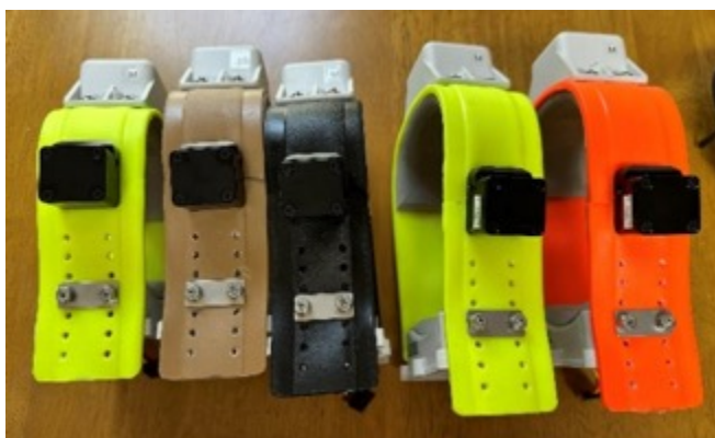
Fig. 11. Lotek LiteTrack Iridium 360+ collars selected as the most suitable collar for dama gazelle. Total collar weight is ca. 400g (exact weight depends on collar circumference, which varies with animal size) and will not exceed 1.6–2.98% of the body mass of a typical adult dama gazelle.
